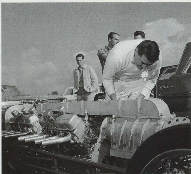
> Not all of Mickey's ideas were successful, but they were always fascinating. At the '62 NHRA Winternationals he ran this twin-engine dragster. A pair of Pontiac V-8s were fed compressed air by a single enormous blower from a GMC industrial diesel.
