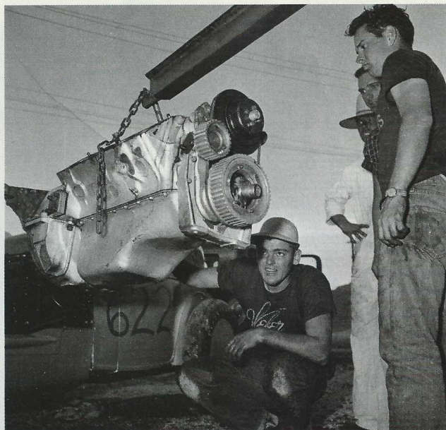
> Above: Bonneville, 1953: A boyish Mickey Thompson (kneeling) pulls one of the engines from his Bantam coupe. The Bantam was twin-engined, with a flathead Merc in front coupled to a Chrysler Hemi. > Below: Mickey with one of the two Hilborn-injected Hemis in his four-wheel drive '58 streamliner at the shop behind his home in El Monte, California.
