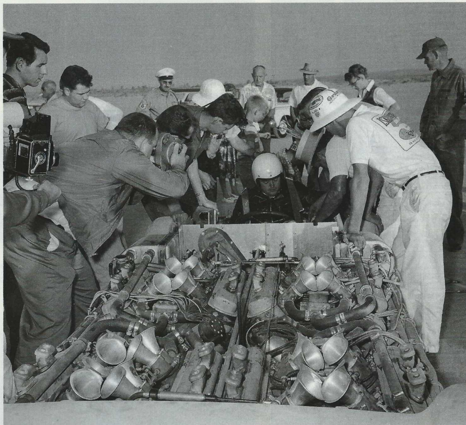
> For Challenger's first year on the Salt, the four Pontiac engines were run normally aspirated. For the record runs in 1960, all four engines received GMC 6-71 blowers.
